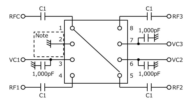
Note: It is recommended to connect the pin directly to the ground, or not to connect the pin to anything.
